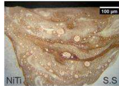
Figure 4. Microstructure of welded sample with 150 \mu\text{m} Interlayer [18].
