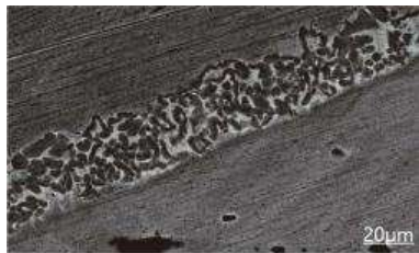
Figure 8. Microstructure of Reaction Layer at 40 A [26].
