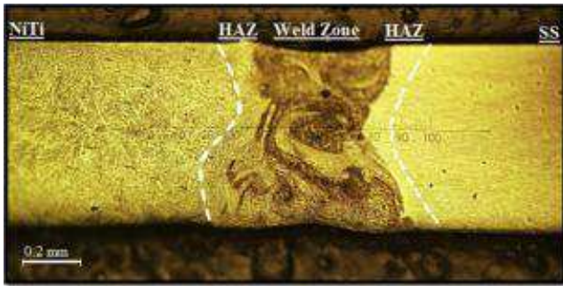
Figure 3. Cross-sectional view of the NiTi to SS dissimilar laser welded joints [17].
